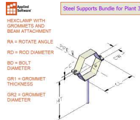
Steel Supports Bundle for Plant 3D
