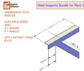
Steel Supports Bundle for Plant 3D
