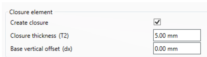
Stairs, Closure Feature: Create Closure check box.
