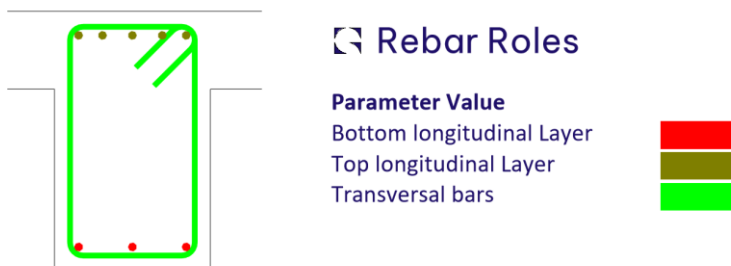
Example of automatically assigned rebar roles
